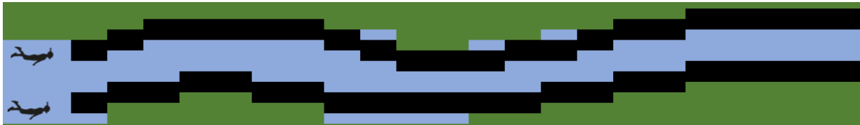
Figure 3 In this example, two surveyors are working in tandem to survey two separate 1 m wide lanes (thick black lines). The middle of this river is not surveyable, and rather than zigzag out from the bank, the surveyors chose to survey a consistent line in the river. For this example, mussels occurred in large numbers and nearly continuously along the edges of the river, so surveying a lane ensured mussels were not double counted. Had mussels been more patchily distributed, a zigzag method would have enabled them to survey more potential microhabitats. If the middle of the river had also been surveyable, adding a third surveyor lane would be advisable for a more complete survey.
